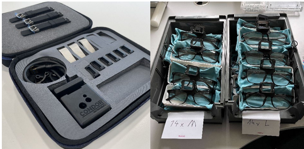
Light loggers, their docking station and wrist straps (left), and 3D printed frames (right)
